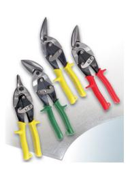
Each style of snips is constructed with comfortable, contoured plastic handles that are color-coded by cutting pattern. The snips are spring loaded for easy self opening, and come with a latch to keep the jaws closed when not in use.
