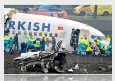
The investigators note that Boeing guidance is that the autopilot and autothrottle should not be used on approach, as they were on the accident flight, if the radio altimeter malfunctioned on the previous flight. It is not stated whether a malfunction was in fact identified on the previous flight.
