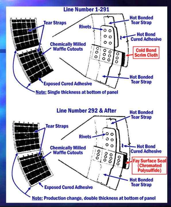
Fuselage Lap Joint Construction:
