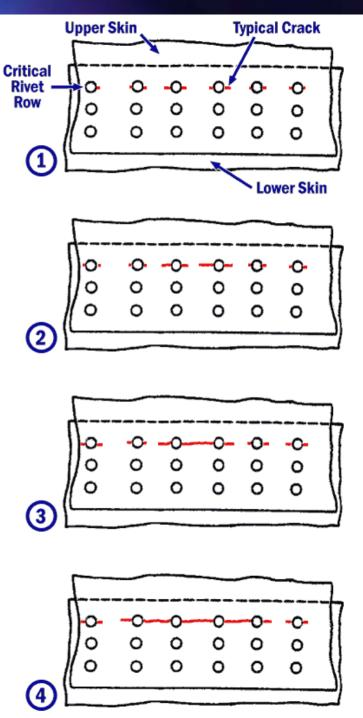
At airplane line number 292, Boeing changed production lap joint process:
