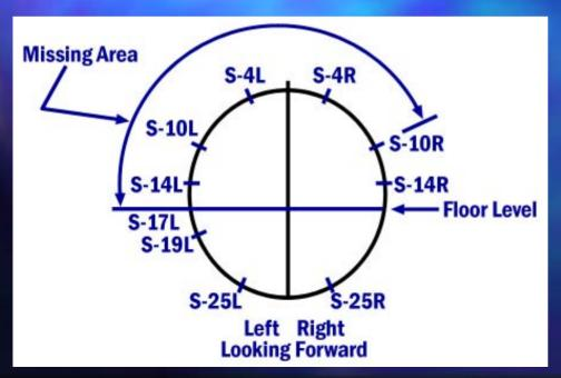
Accident was caused by pressurization related cyclic fatigue of fuselage lap joint:
