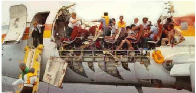
Miraculously, the pilot managed to land the plane on the island of Maui, Hawaii. One flight attendant was swept to her death. Multiple fatigue cracks were detected in the remaining aircraft structure, in the holes of the upper row of rivets in several fuselage skin lap joints.
