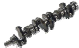
When crankshafts in **higher-horsepower Lycoming engines failed** from 2000 to 2002, Lycoming blamed Interstate for **improperly heat-treating** the blanks it forged. However, the 2005 verdict determined that Lycoming had **changed the recipe for the alloy** used to make the crankshafts by adding vanadium. The vanadium made the steel easier to work with, but it also weakened the end product.
