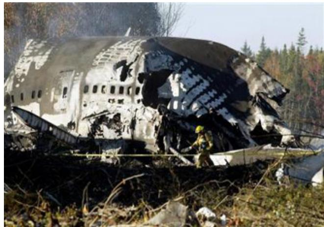
As a result the airplane was traveling about 30 knots (35 miles an hour or 56 kilometers an hour) slower than the 160 knots that would have been required for a safe takeoff with the load it was carrying.
