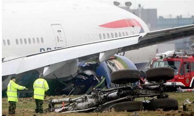
The Air Accidents Investigation Branch said the fuel leak did not cause the accident but **could have had serious consequences** if the Boeing 777 had caught fire after slamming into the ground hundreds of meters from the runway. The AAIB also **ruled out an intake of ice** into the engines or a **bird strike** as causes of the crash.
