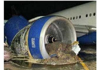
When they took apart the engines, investigators found evidence **on pumps that the engines had been starved for fuel** in the moments before the crash. That led them to conclude that the fuel supply had **become blocked** somewhere between the plane's tanks and its engines.
