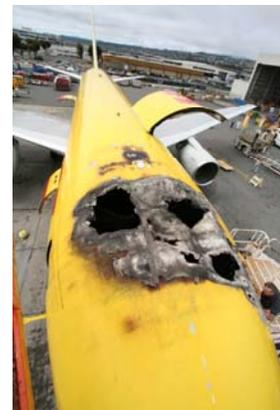
The primary location of the fire was outside the cargo hold in an area just aft of the cockpit. The fire was extinguished by San Francisco Airport Rescue and Fire Fighting, but not before causing substantial damage to the aircraft. The flight crew of two, who were preparing to start the engines when the fire broke out, escaped from the aircraft without injury.
