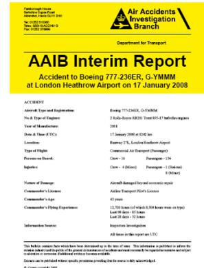
The report states in summary that the investigation has shown that both engines suffered from restricted fuel flow **"most probably due to ice within the fuel feed system."**
