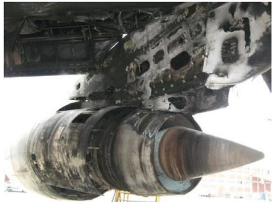
While exiting the runway the crew received a fire indication for the inboard starboard Pratt & Whitney JT9D engine. Attempts to extinguish the fire were unsuccessful and the crew shut down the engines and ordered an evacuation.
