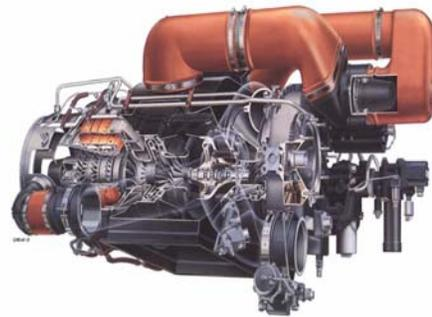
Investigators are still trying to understand the mechanism for the failures - experienced by at least two A330 operators on the ground - but the [European Aviation Safety Agency](#) states that **collapse of the APU's drive-end bearing** appears to be a preceding event.
