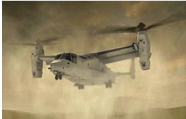
According to the Judge Advocate General Manual Investigation report -- obtained by Military.com through a Freedom of Information Act request -- **a leaking hydraulic line** spilled fluid onto the engine's infrared suppressor section, sparking a blaze that nearly consumed the aircraft in the November 6, 2007 incident.
