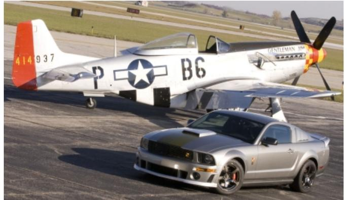
There are a number of changes to this themed Mustang, such as the black chrome wheels, ROUSH vent pod gauge with a boost gauge, and ROUSH 6-piston brakes for extra stopping power. The six-piece ROUSH aero body kit will help the car stand out in the crowd.
