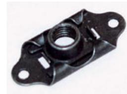
Now, tens of thousands of others **lack an important coating of cadmium**. That nearly invisible coating is important because it prevents the stainless steel nutplate from reacting with the airplanes aluminum, which can **lead to corrosion**.
