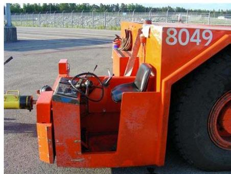
Although the Schopf 356 tractor had been moved a short distance, **it remained out of the pilots' field of vision**. SHK says that, while the pilots read the normal checklist after engine start, it "did not contain any point" concerning a "clear signal" - a thumb-up gesture showing an aircraft is clear to taxi.
