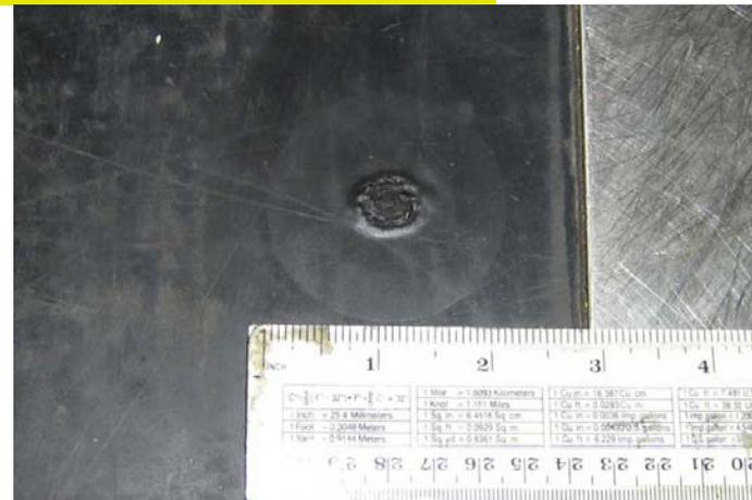
Recently a MagLite 6V 2.5 AH rechargeable Flashlight was inadvertently left switched on and standing on its lens assembly. After a short period of time a burning plastic smell was detected and traced to the flashlight. The lens area of the flashlight had become overheated and scorched the vinyl bench-top. The incident highlighted a significant fire hazard; particularly had it gone unnoticed or occurred after hours.
