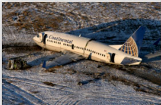
Continental Flight 1404 was taking off from Denver at 1818h local time when pilots **lost directional control** as the aircraft reached approximately 100kt airspeed. The aircraft departed the left side of Runway 34R, coming to rest in a drainage basin and catching on fire. All 115 passengers and crewmembers escaped, though 41 were injured.
