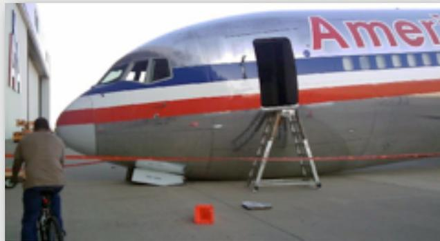
It now appears that mechanics in the cockpit pulled the lever that retracts the landing gear, **not realizing** that other mechanics failed to put a pin in the gear to prevent it from actually retracting while the plane was on the ground.
