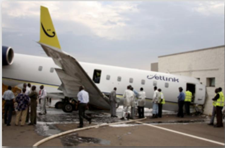
Jetlink reported, that the airplane **was taxiing in**, when the aircraft impacted the pavilion of the VIP lounge **nose-first with engines at high power**. All passengers could leave the airplane on their own, the airline however believed that one female passenger passed away in hospital.
