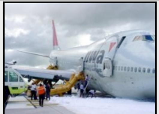
According to a probable cause report by the NTSB, the plane's flight crew **failed to confirm** there were five green landing gear indicator lights, as stated in the checklist. The crew instead **made general comments** about the lights, such as "got em all," the report states.
