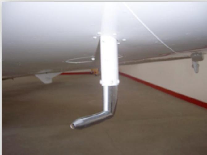
The incident has prompted the FAA to issue a Information for Operators (InFO) advisory informing aircraft operators of the potential for pitot-static system malfunctions **after an aircraft is repainted**.
