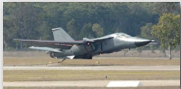
They had IPs trying different solutions in the simulator. Finally it was decided we'd fly the approach at about 1.5 meters off the ground for a few hundred meters with the gear up and the tail hook dragging along the ground.
