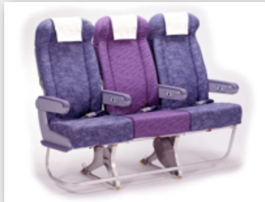
The American Airlines 737-800 was only 8 years old, and it was equipped with **newer 16G seats**, which are designed to withstand forces up to 16 times the force of gravity in a crash.
