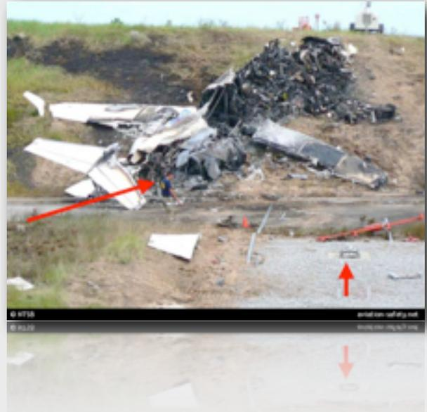
According to the Safety Board, the accident airplane’s tires **lose 2 percent of pressure every day**. The full inflation of 219 psi drops to 185 after eight days and after three weeks reaches 140 psi, the level estimated in the accident airplane.
