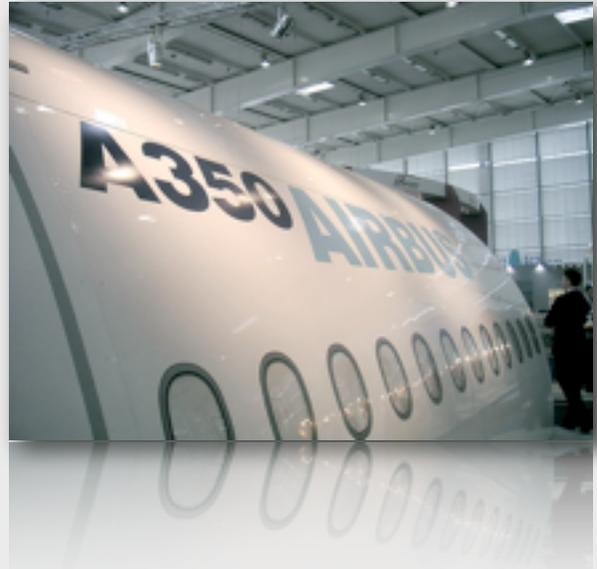
The A350's fuselage and cabin physical mock-up is being assembled at Airbus's Hamburg plant, with the front fuselage so far having been constructed. "In the coming months the whole fuselage will be built - we have already used it a lot last year for testing design, assembly processes, tools and jigs," adds Evrard.
