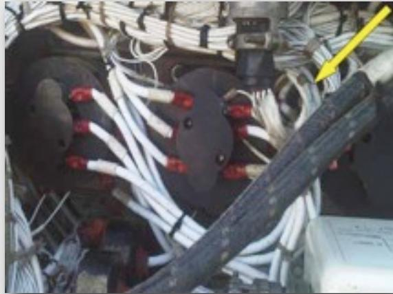
They applied ground power to the jet. Then, with meter in hand, the AE3 began reading for power at all the relay terminals. Unfortunately for him, this meant sticking his hand next to a **nest of wires and terminal lugs**. As he reached into the panel to read for power, he brushed up against a live wire, which jolted him immediately with a painful shock. The two secured power quickly and went back to the shop.
