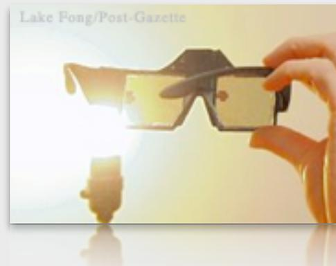
Together they identify glare and react by applying more sun filtering to the LCD in that area of the lens, even as the wearer turns his or her head. In practice, wearers see a dark non-opaque spot hovering over the sun, or any other source of glare that exceeds a programmed threshold. The prototype is still relatively bulky and may challenge popular fashion sense, but the concept has earned attention (and funding) from the Air Force.
