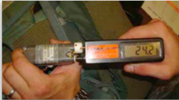
The cautions dealing with the probes are clearly explained as, “Failure to do so will result in an inadvertent firing of the PHSRU.” However, the reason for only using FLUKE 77 series multi-meters is not totally clear. Here’s the explanation. In the 1990’s, the CONAX Florida Corporation manufactured a Battery Voltage Tester that mitigated the risk of contacting probes (see photo). It was subsequently authorized for Navy use and many work centers started using them.
