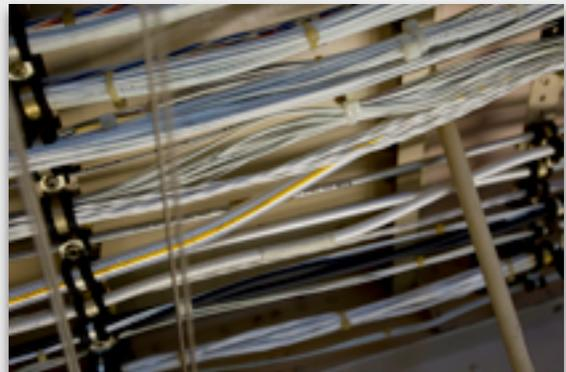
The leads may be improperly identified or missing labels, according to the FAA's proposed airworthiness directive to remedy the situation.
