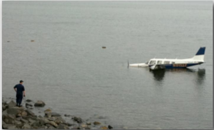
The crash occurred on Aug. 12, when the pilot and mechanic of the Piper Cherokee were taking the plane on a test flight following maintenance to the aircraft. Upon approach to the runway, the pilot reported that the throttle control became unresponsive, resulting in a partial loss of power, according to the report.
