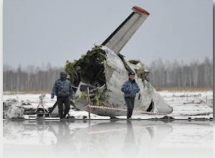
Although a technician had examined the aircraft [from the ground](#), says the Interstate Aviation Committee, the critical surfaces [could not have been seen](#) without the aid of a ladder or elevated platform. The ATR's crew arrived at 06:30 on 2 April but, although the captain performed a walk-around, he similarly [did not pay sufficient attention](#) to the presence of ice deposits on the wing and stabilizer - despite the de-icing carried out on aircraft parked on adjacent stands.
