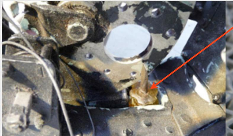
The report, written by safety investigator Alan Moselen, found the crash was the [result of design flaws in the plane](#) that led to a screwdriver getting stuck in the elevator controls of the plane during a "slow roll" maneuver.
