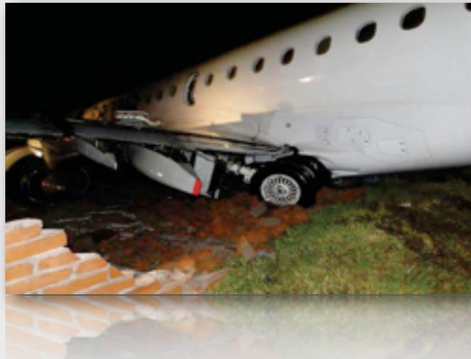
Ecuador's Junta Investigadora de Accidentes says the pilots attempted five times to reset the flaps, but that the slats would not deploy and the flaps would only move to position 2.
