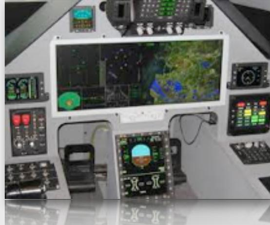
Collins's advanced technology center. Shapiro had assembled the group to gather input on an advanced technology project to simplify the autopilot or “autoflight” modes that accompany flight management systems. A legacy airliner or business jet can have nearly 40 distinct autoflight modes for lateral, vertical or airspeed maneuvers.
