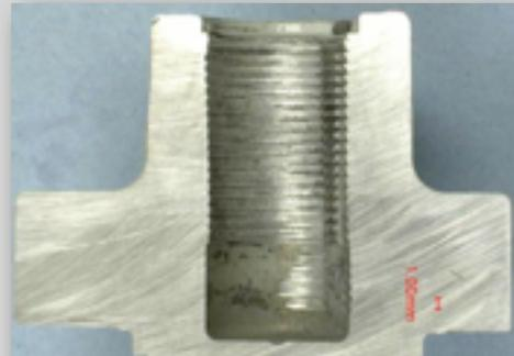
Heavily worn threads caused by use of an unapproved compound in a threaded rod end installation.
