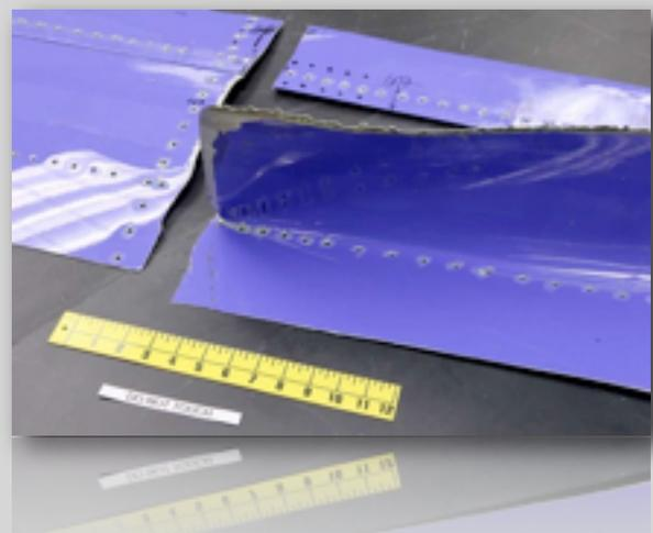
"Investigators determined that ATS [failed to follow proper procedures](#) for replacing the fuselage skins on these aircraft. FAA investigators also determined that ATS [failed to follow required procedures for placing the airplanes on jacks and stabilizing them](#). All of the work was done under the supervision of Southwest Airlines, which was responsible for ensuring that procedures were properly followed," says the agency.
