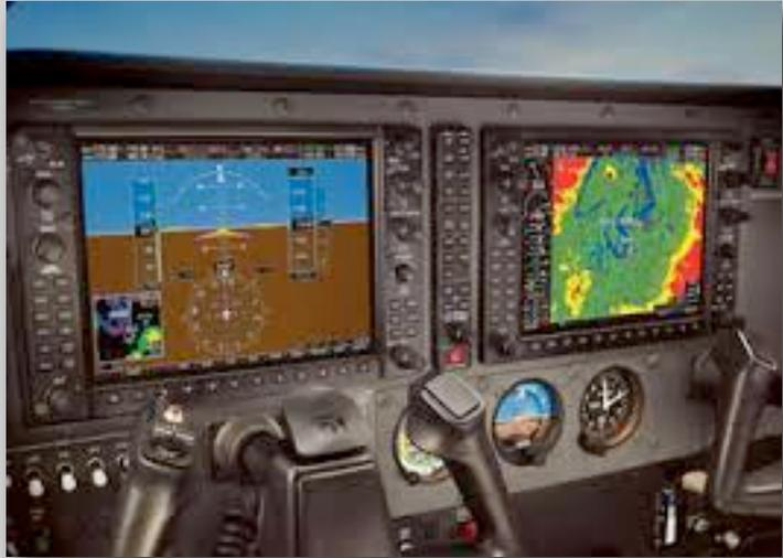
In recent years, the cockpits of many general aviation aircraft have undergone a transition from conventional analog flight instruments to digital-based electronic displays, or “glass cockpits.” While these “glass cockpits” represent a significant change and potential improvement, they also represent challenges for pilots in the GA community.
