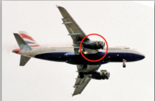
The design of the fan cowl door latching system, in which the latches are positioned at the bottom of the engine nacelle in close proximity to the ground, increased the probability that unfastened latches would not be seen during the pre-departure inspections.
