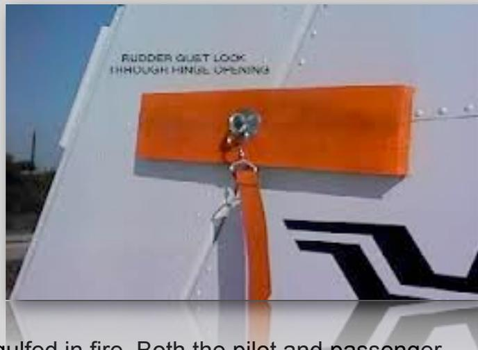
While it could not be determined who was at the controls of the airplane during the accident flight, **both pilots should have noted the installation** of the rudder gust lock either during a preflight inspection or during a pre-takeoff check of the flight controls.
