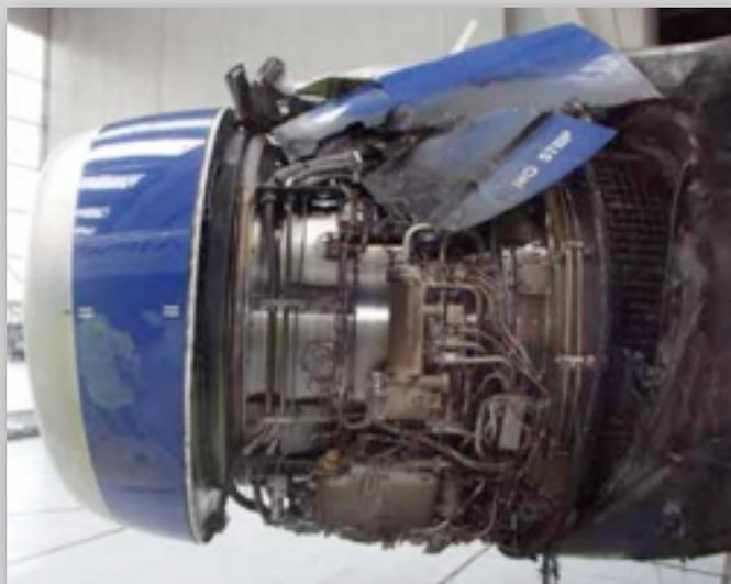
This condition remained undetected during the exterior walk-around preceding departure, leading to air scooping and subsequent cowl separation. Airbus is currently working [on a new design solution](#) for the A320 family fleet, improving the identification of any fan cowl door not properly closed and latched. That modification is expected to be the subject of an Airworthiness Directive (AD).
