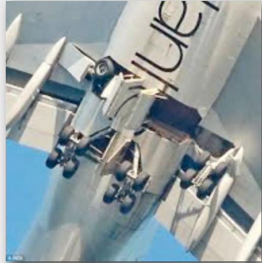
In its analysis of the event the Air Accidents Investigation Branch found that the aircraft had undergone replacement of the actuator on the right wing main gear [the night before the flight](#).
