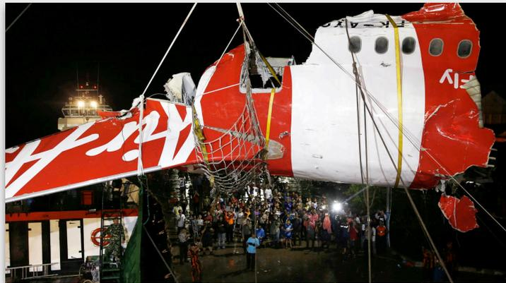
said that a solder joint in a circuit board could have led to rudder problems that caused the crew to try to fix the autopilot by re-setting a circuit breaker. The crew eventually lost complete control of the airplane.
