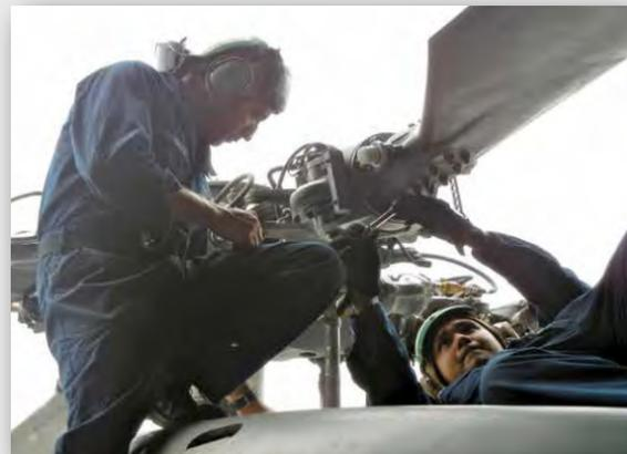
The Phase “D” inspection is a challenge because it entails removing all main rotor blades and spindles for subsequent rebuild and replacement. This task is difficult ashore and even [more challenging while underway](#).
