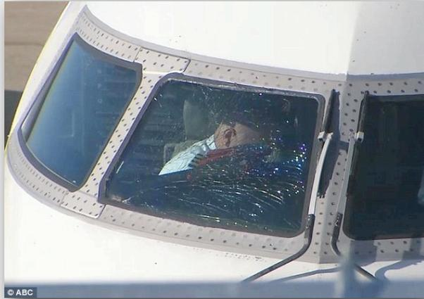
At three plies thick, glass windshields are designed to protect against bird strikes; de-ice from minus 50 degrees; resist fogging and provide exceptional optical qualities.
