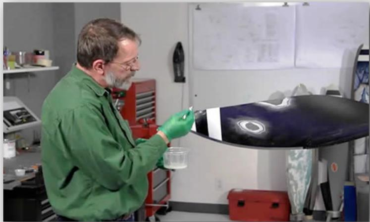
"As with aluminum blades, composite blade damage can be evaluated and often repaired on-wing by a certified Airframe and Powerplant (A&P) mechanic using information provided by Hartzell."
