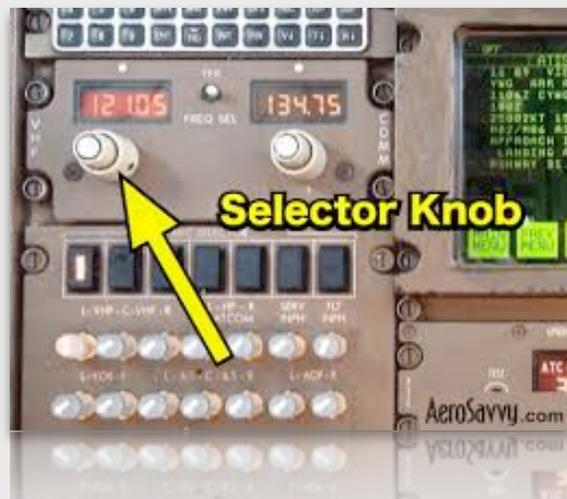
A few examples of common causes of unintentional selections include mechanical interference between two concentrically centered knobs; pilots accidentally rotating two knobs at once as a result of finger positioning errors and/or finger slippage; and pilots inadvertently selecting the wrong knob and subsequently failing to make corrections because they did not detect the error.
