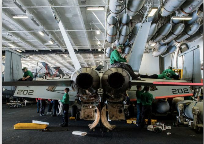
California. The pilot landed injury-free at China Lake, but the plane wasn't so lucky. It suffered burn damage to its starboard engine door. There were also burns on the engine exhaust nozzle skin, wiring, and fire emergency equipment, and so they needed to be replaced.
