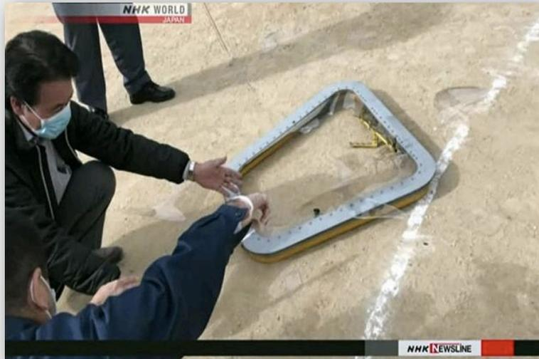
"A thorough inquiry determined that the incident was caused by **human error**," 1st Marine Aircraft Wing officials said in a statement released Sunday. "The window in question is designed to be removed in order to assist pilot egress in an emergency situation. **The appropriate procedures for ensuring the window was secured were not correctly followed.**"
