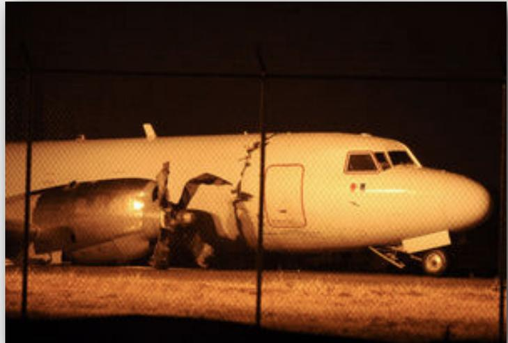
A **large crack** could be seen separating the cockpit from the plane's body and the propellers were destroyed.
