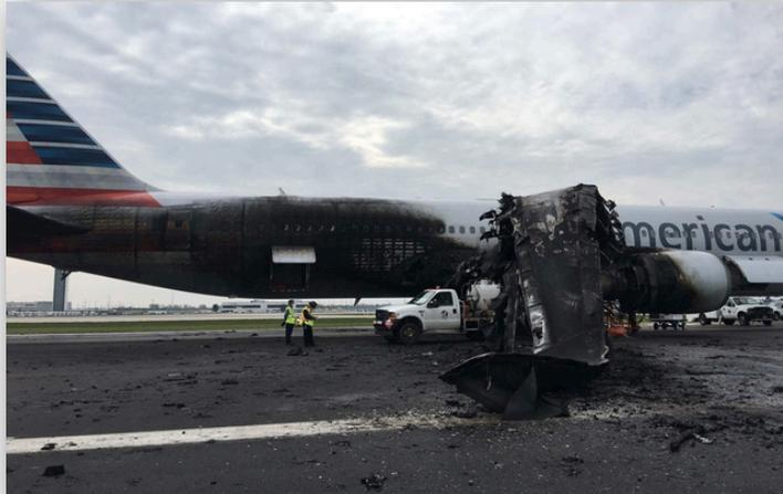
The failed turbine disk was recovered in four pieces, one of which weighed 57 pounds and was found more than a half mile from the airplane. Through extensive examination of the disk fragments at the NTSB lab in Washington investigators determined there was a [subsurface defect in the disk at the time of manufacture](#). Because of the nature of the defect and the [limits of inspection methods](#), the NTSB concluded the defect was [likely undetectable](#) when the disk was produced in 1997.
