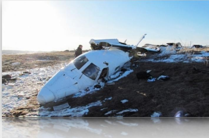
descent from FL 210 **to save fuel**, then began descending at just 800 fpm instead of his planned 1,500 fpm. The descent rate subsequently reached 2,500 fpm, but the airplane crossed the initial approach fix (9.7 nm from the runway threshold) 1,500 feet high and 100 knots faster than its recommended approach speed, overshooting the final approach course before correcting.
