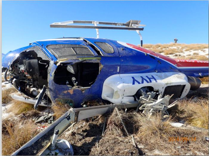
When the pilot approached the landing site, the rate of descent suddenly increased, so he "increased the power to go around," the report said. That's when the helicopter struck the ground with the landing gear and the main rotor blades, and rolled onto its left side.
