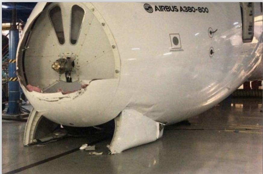
Occurring at an Emirates maintenance hangar at Dubai International Airport, the accident has left the aircraft with a torn/crumpled fuselage and structural damage.
