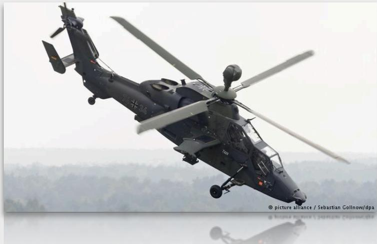
The Tiger helicopter had been serviced by Airbus team which [apparently forgot to set the blades' airflow angle correctly](#). As the helicopter was flying roughly 155 mph at an altitude of 1640 ft over the Gao desert, the Tiger's autopilot switched itself off believing that it had recognized a manual override, leading the helicopter to tilt forwards abruptly. Once the vehicle had started to descend, parts of the aircraft broke off, including the main rotor blades.
