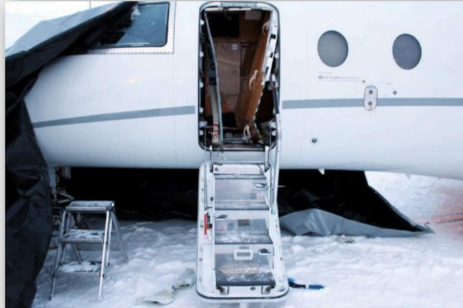
In a safety information bulletin (SIB) issued on 12 February, the European Aviation Safety Agency (EASA) identifies "an excessive differential pressure between the inside and the outside of the aircraft", as the root cause of the problem.
